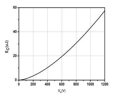
Fig.7-Capacitance Stored Energy
